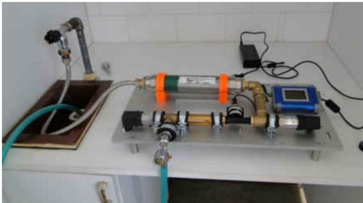
Figure 2 Developed device for regulating water pressures in the flow
