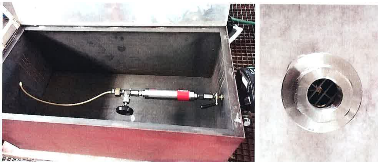
Picture 2 IPS RedLine in the test cabinet and during distance measurement.
