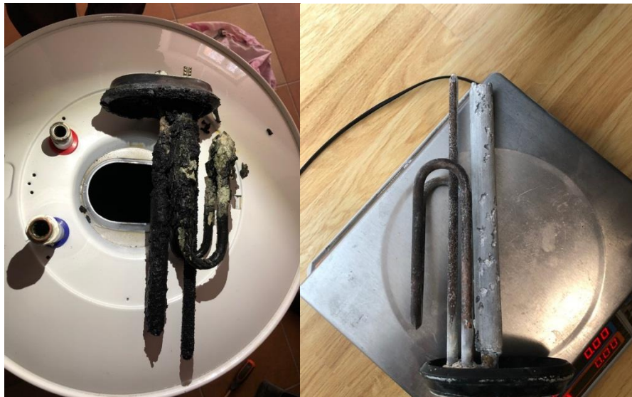
Fig. 2 Bojler heating coil before and after cleaning
