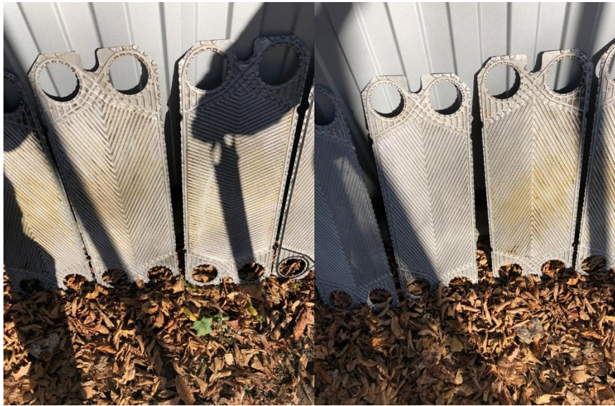
Fig. 1 Heat exchanger plates cleaned and ready for test 12.11.2018
