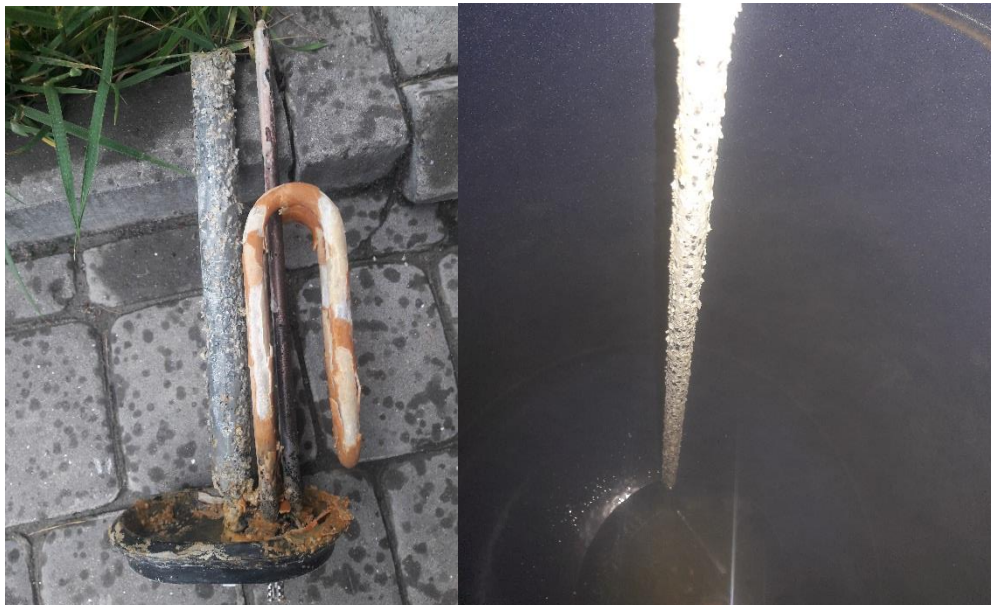
Fig. 5 Bojler heating coil without treatment (1,8 m 3 ) 15.05.2019
